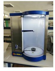
The 3D Laser Scanner is a measuring and analyzing instrument of morphological data of the samples, providing info such as volume, weight, dimensions, etc. The volume analyzer is suitable for many different kind of products.
